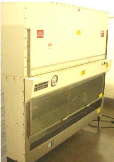
The Class II Laminar Flow Biological Safety Cabinet, or the Biosafety Cabinet, combines product, operator and environmental protection. It was developed to provide protection from diverse types of biohazardous material. The biosafety cabinet is similar to the conventional fume hood in providing protection for the operator. It differs from the conventional fume hood by also offering protection for the work in progress and the environment.
